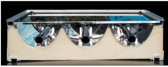
This demonstration cross-section shows the insulation, glazing, and concentrating parabolic collector configuration used in the Winston Series CPC collector. Photo: Solargenix Energy, LLC
